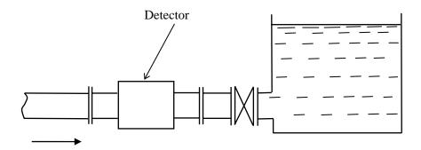
Figure 4.11 Detector with sufficient head pressure at downstream outlet
